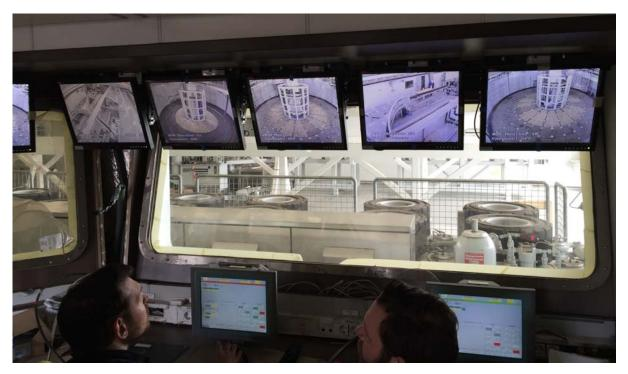
Integrated Cable Handling Control Stations
